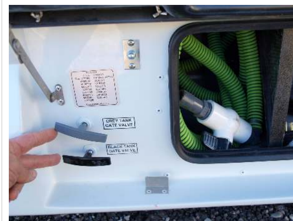
Driver's side front access door showing tank dump valves and waste water hose
