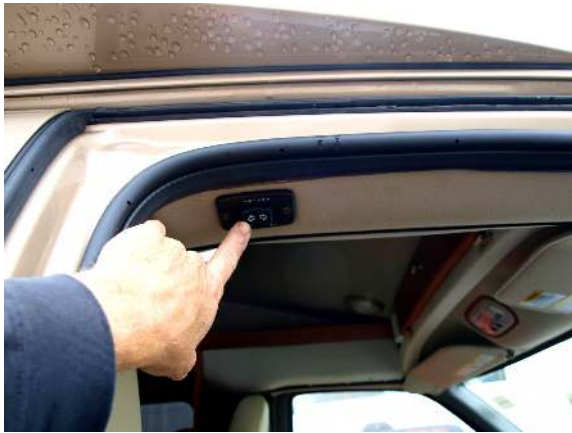
Awning power switch
