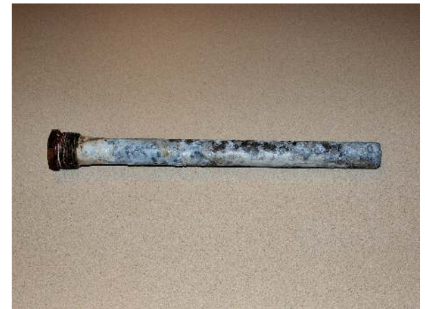
Water heater anode with some corrosion, but probably cleanable and usable for another year.
