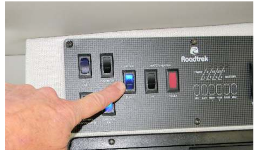
Water pump switch on (blue indicator light lit)
