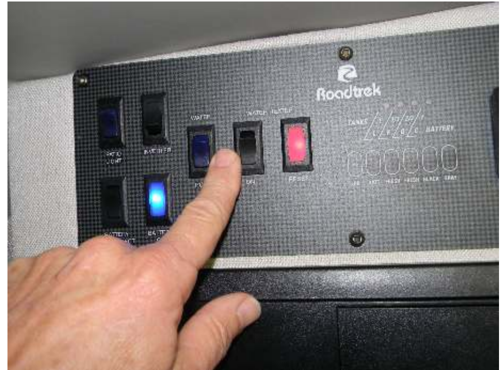
Water heater switch and red indicator light
