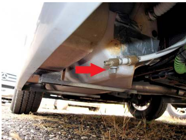
Fresh tank drain under driver's door
