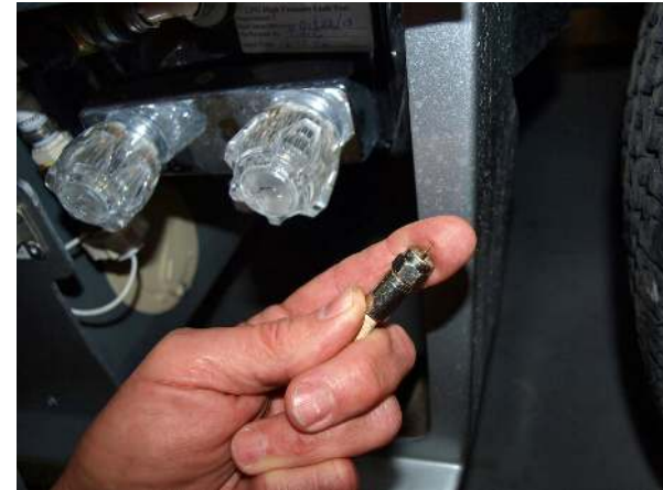
Coaxial TV connecting wire with screw-on end
