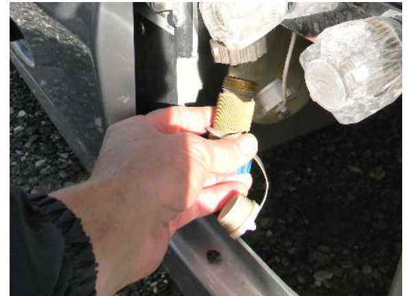
Attaching pressure regulator to city water fill location
