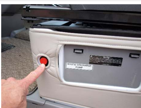
Macerator button on base of driver's seat
