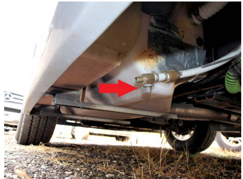
Freshwater tank drain valve
