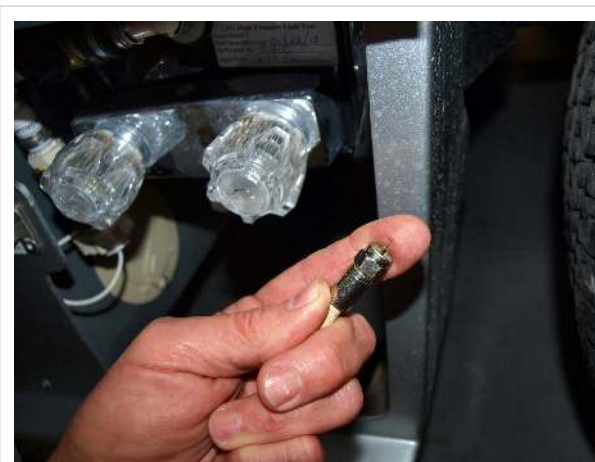
Coaxial TV connecting wire with screw-on end
