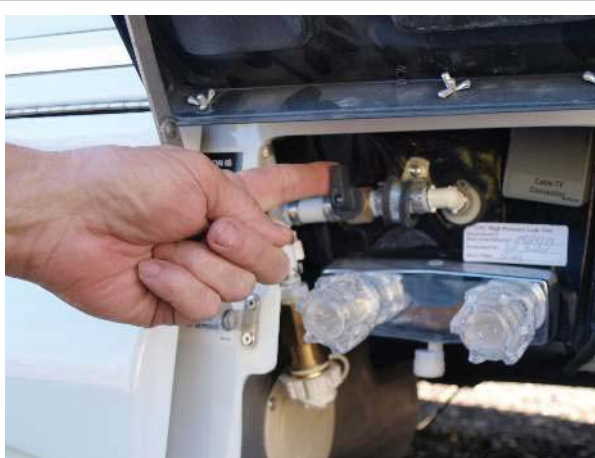
City water connection valve, shown closed
