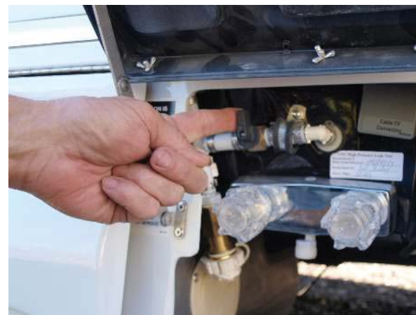
City water valve, in small compartment in front of driver's side rear tire
