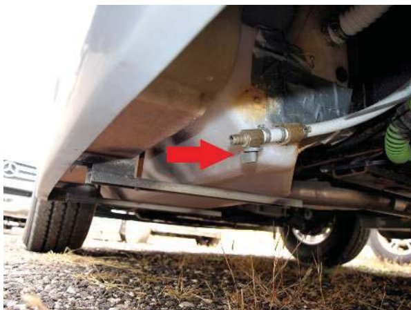
Fresh tank drain under driver's door
