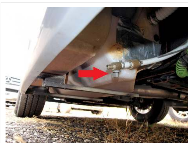
Fresh tank drain under driver's door
