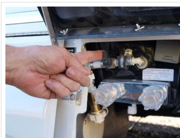
City water valve, in small compartment in front of driver's side rear tire
