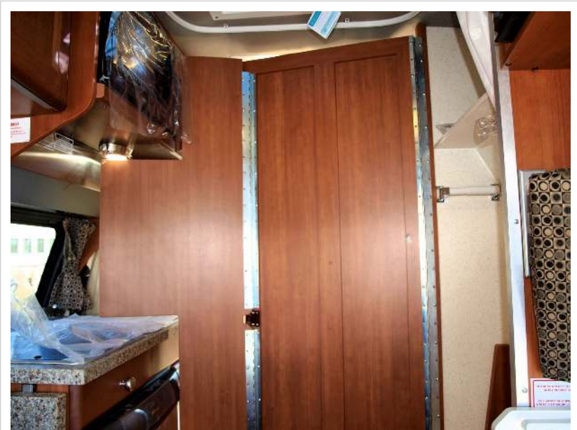
Door extended into privacy position
