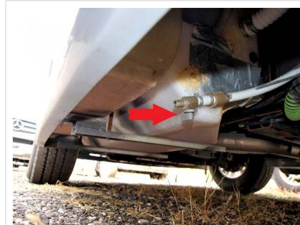
Fresh water tank drain, under driver's doorstep
