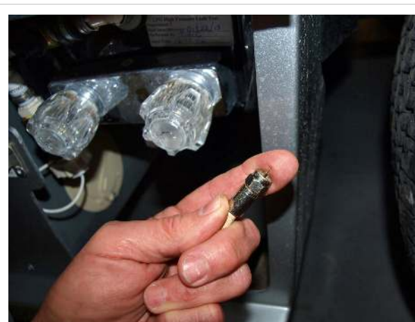
Coaxial TV connecting wire with screw-on end
