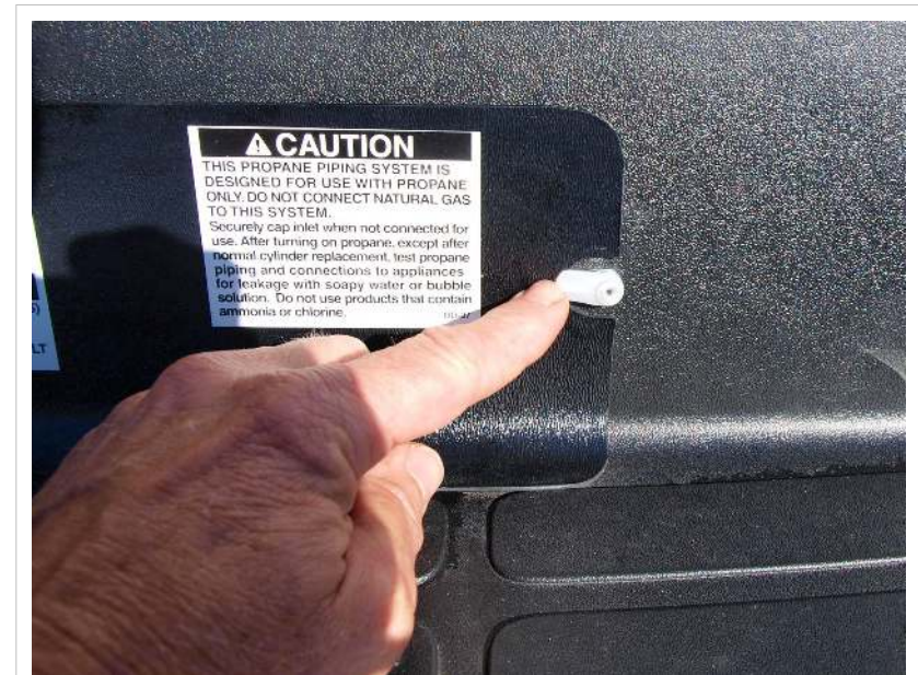
Propane access cover
