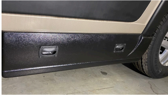
The entire waste management station is concealed behind a lower sidewall skirt.
