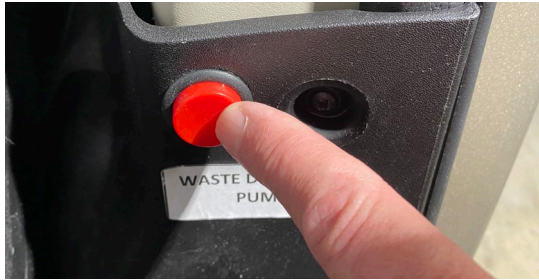
Touch a button to activate Macerator pump
