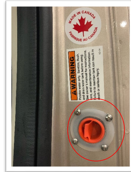
The gravity feed to fill the freshwater tank is in the B pillar of the driver's side door frame.
