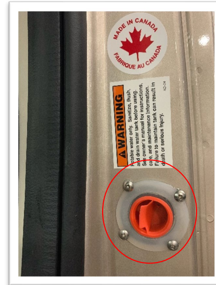
The gravity feed to fill the freshwater tank is in the B pillar of the driver's side door frame.
