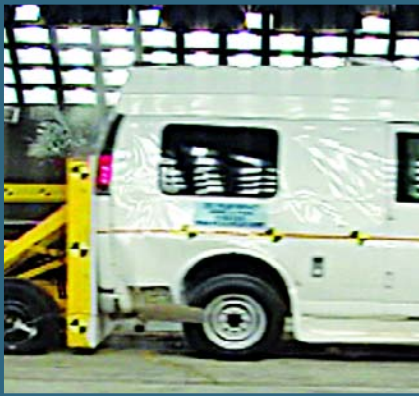
This photo shows the rear impact test. The test vehicle was impacted by a moving barrier at 30-mph (48 km/h). The entire fuel system was then inspected for leakage. Our test vehicle did not leak any fuel.
