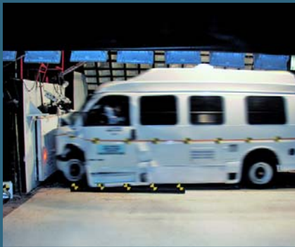
For frontal impact testing, the test vehicle impacted a fixed barrier at 30-mph (48 km/h). Again our test vehicle did not leak any fuel.
