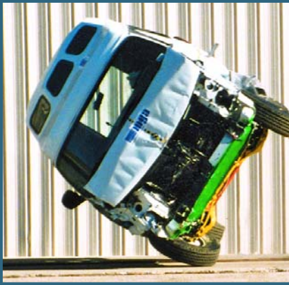
Dynamic rollover testing is intended to reduce deaths and injuries from occupants and their appendages not remaining within the passenger compartment during rollover accidents.
