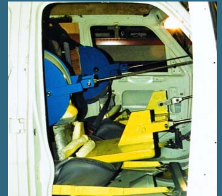
These 2 photos depict simultaneous seat belt pull testing and seating system testing. Seat belt testing confirms proper seat belt location and minimizes the possibility of anchorage failures. Seating system testing verifies the integrity of the seats, their attachments, mounting hardware and installation.
