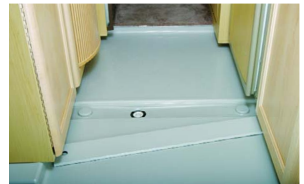
A removable cover in Chevy based Roadtreks reveals a trough with a drain that spans the lowered floor and prevents water from leaving the shower area.
