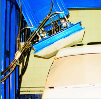
Roof crush resistance testing is intended to reduce deaths and injuries from roof crushing during rollover accidents.
