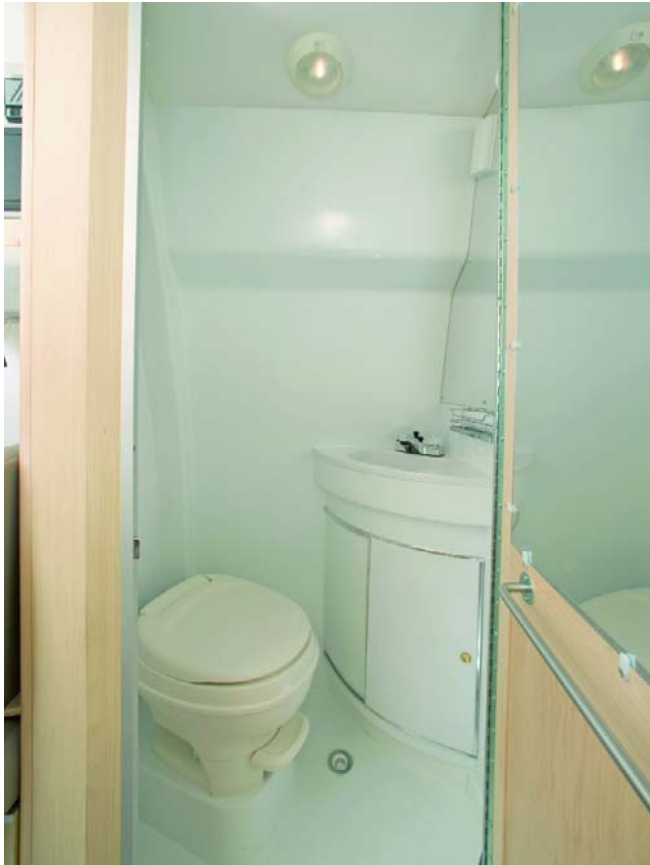
The 210's optional permanent bathroom features complete privacy, toilet, vanity sink with storage cabinet, mirror and 110V receptacle. The shower can be used as a sit-down shower with the door closed or used in the aisle as a stand-up shower.
