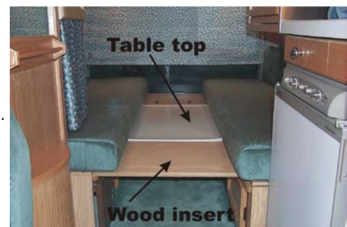
Picture B-P10: Placement of support pieces for the king size bed (Popular).
