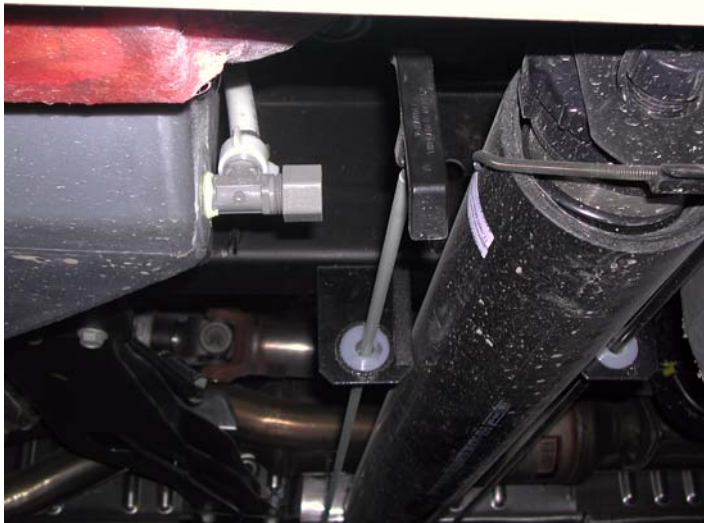
Picture G-P20: Location of the exterior freshwater tank drain.
