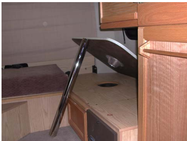
Picture B-P7: Storage location of dinette table, showing placement of the table base receptacle (Versatile).
