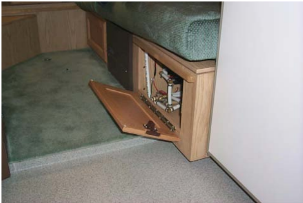
👉 Picture G-P14: Location of the access door for the tank selector valve.
