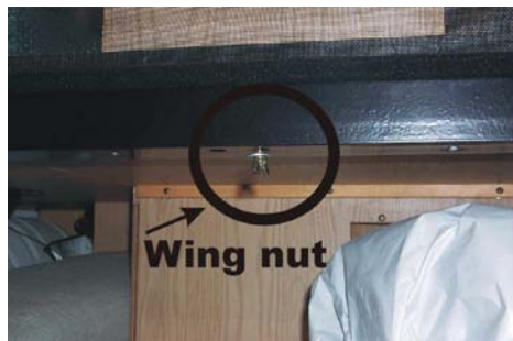
Picture B-P9: Wing nut attaching the night table, needs to be accessed from the rear storage area (Popular).
