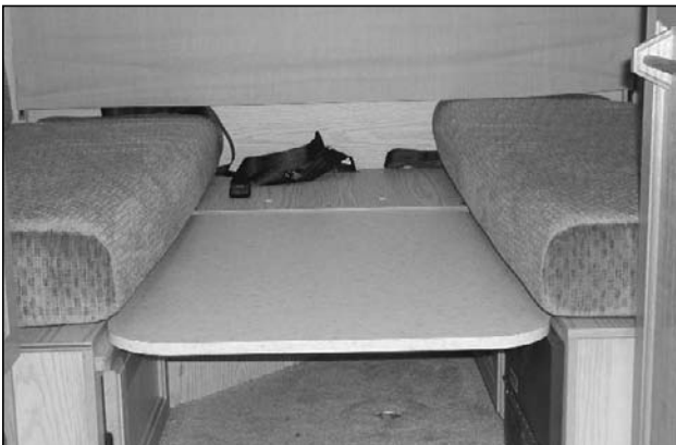
Picture B-P13: Placement of dinette table used as the center support for the double bed, (Versatile model).
