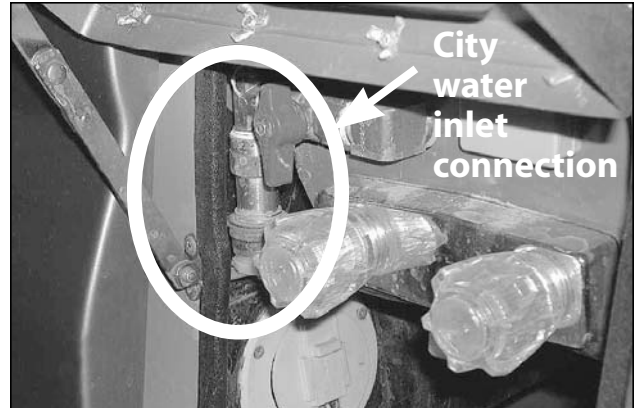
Picture G-P3: Location of the city water inlet connection.
