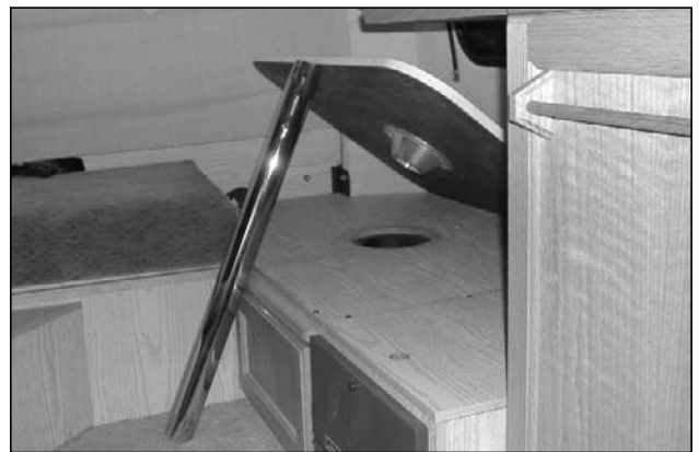
Picture B-P8: Storage location of dinette table, showing placement of the table base receptacle, (Versatile models).
