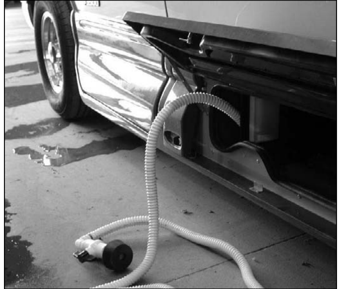
Picture G-P10: Macerator hose location
