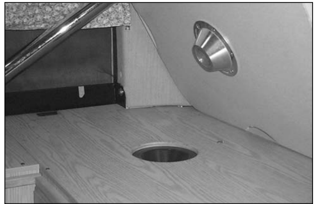
Picture B-P6: Storage location of dinette table, showing placement of the table base receptacle, (Popular models).
