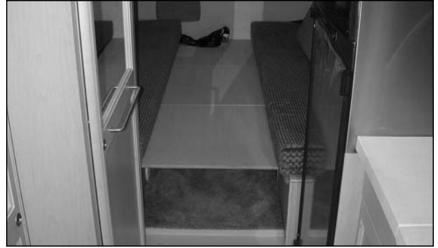
Picture B-P10: Placement of supports for the King size bed, (Popular Model).
