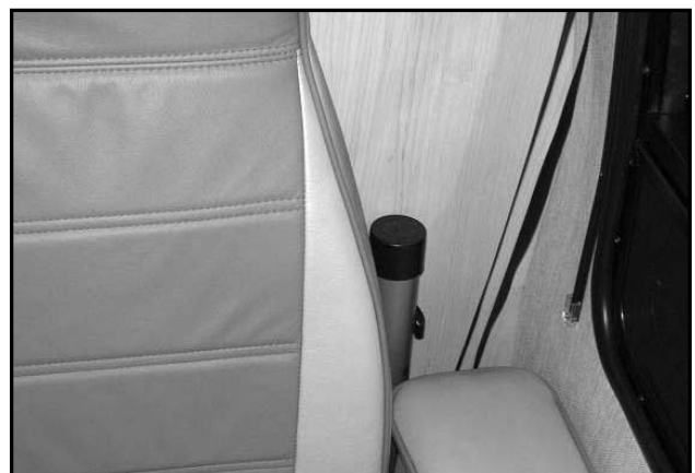
Picture B-P4B: Cloverleaf table leg is stored beside the driver side lounge or captain seat. (Versatile model).
