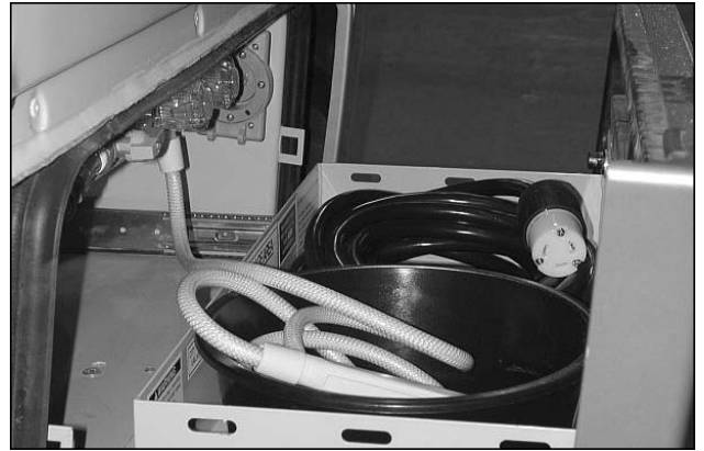
Picture G-P19: Outside shower and shore power connection. Shower hose storage when Motorhome is parked.
