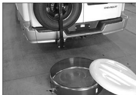
Picture B-P46: Remove the chrome ring and fiberglass disc.
