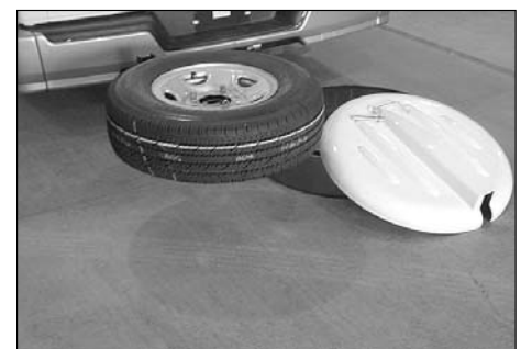
Picture B-P47: Remove the catch pin and the lower carrier to remove the spare tire.
