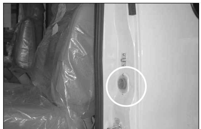
Picture G-P9 : The water fill for the external fresh water tank, (located at driver’s side front door post).
