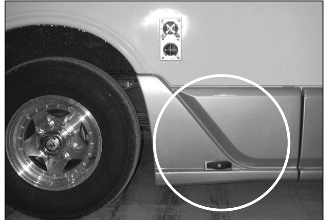
Picture B-P42: Auxiliary battery(s) compartment.
