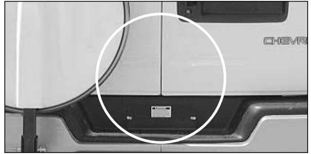
Picture B-P39: Propane access panel.
