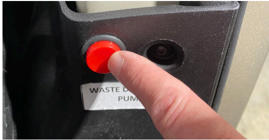
Touch a button to activate Macerator pump
