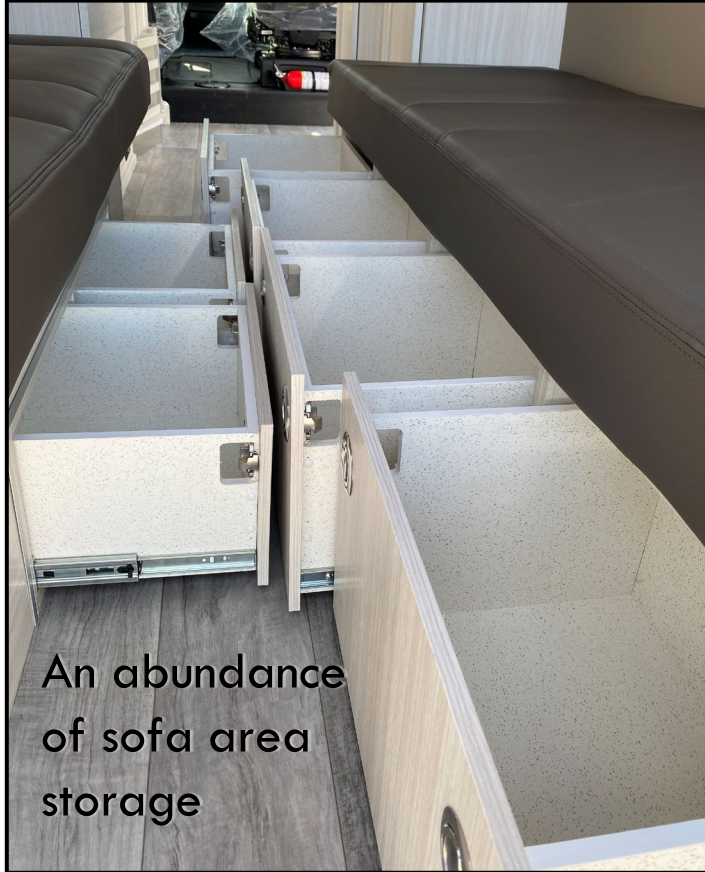
Base cabinets are precision docked into notches in the subfloor. This extra step keeps cabinets "rock solid" in place preventing fatigue from hard braking and rough road travel.
