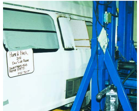
These photos depict side crush resistance testing which is intended to simulate the vehicle impacting a utility pole at a perpendicular angle.
