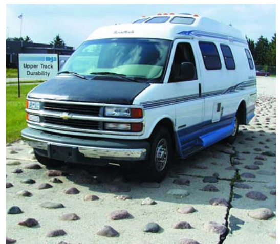
"Automotive manufacturer" style durability testing allowed us to quickly identify and implement numerous design improvements which would otherwise only become apparent during the normal life of the first vehicles built and sold.
